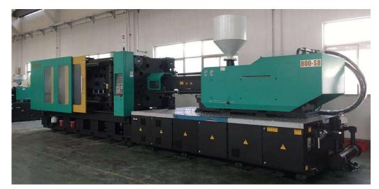
Large parts such as Bumper & Instrument Panel are handled by the China Tryout Center's 1600-3500mm molding machine.
